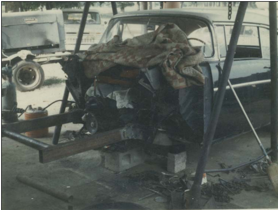
Figure 18: '57 Chevrolet during Construction of Front Axle Note the engine moved back 11 inches and new frame.
