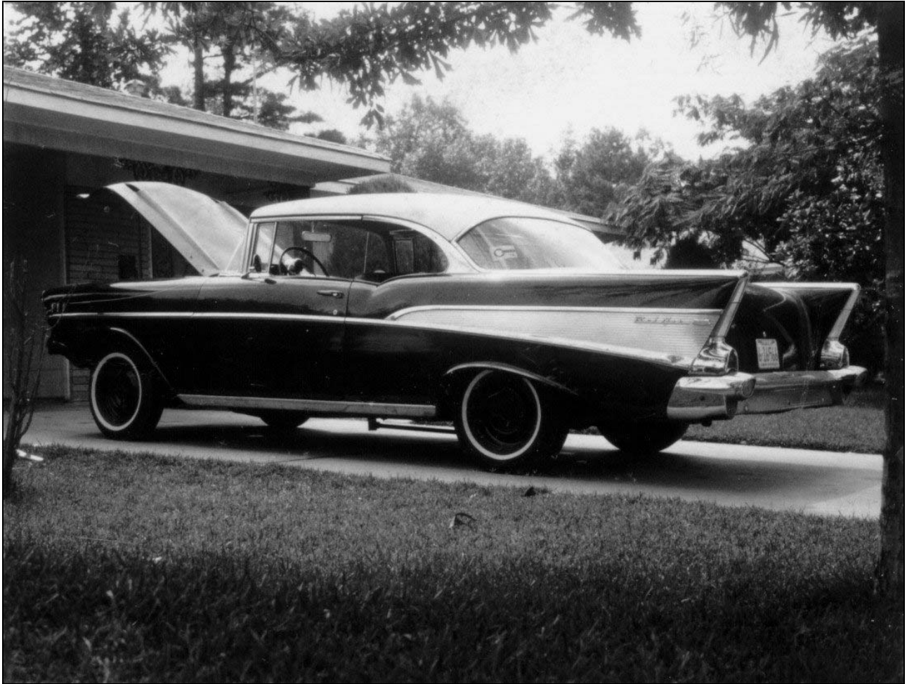
Figure 10: '57 Chevrolet Showing Volkswagen Tires and Traction Bars The Volkswagen tires were used for a while in the front. They did not aid traction because the front end was down lower. The traction bars were made by Mr. Woolsey and helped protect the rear springs. Note how the hood was held up.
