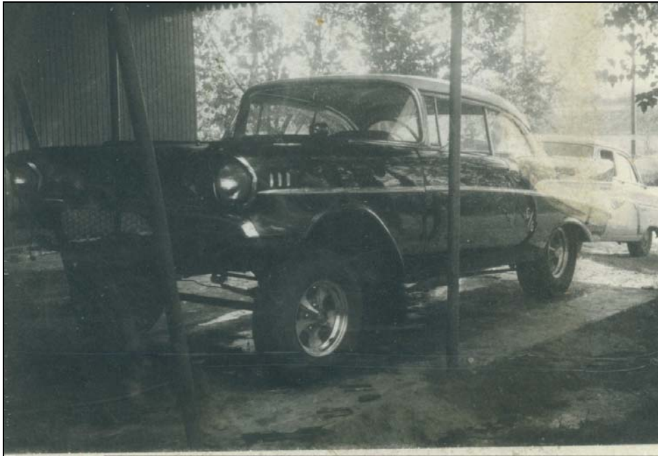
Figure 19: Completed Straight Axle Assembly Except for Axle Brace The front springs and gap behind the grille are shown.
