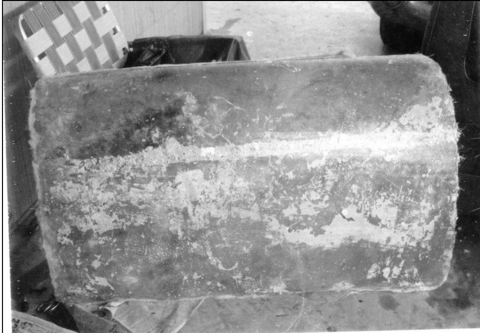
Figure 16: Fiberglas Door after Removal from Mold The outer side of the fiberglas door is shown. At this time, the door side weighs only two pounds.
