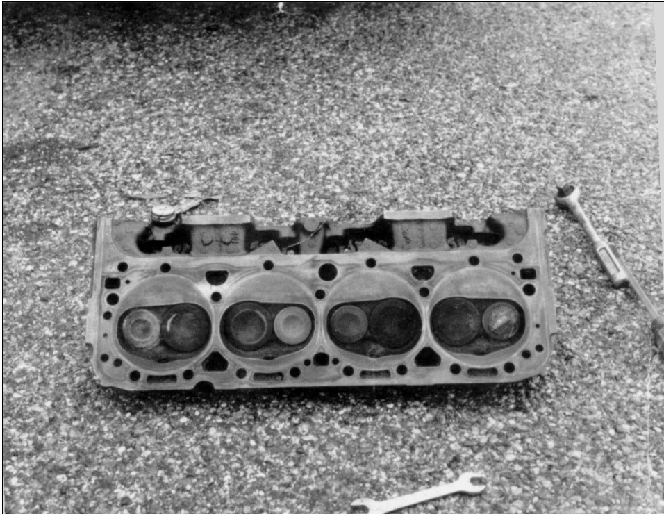
Figure 8: '57 Chevrolet Head One of the removed 2.02 is shown. Note quench area of early 2.02 head.
