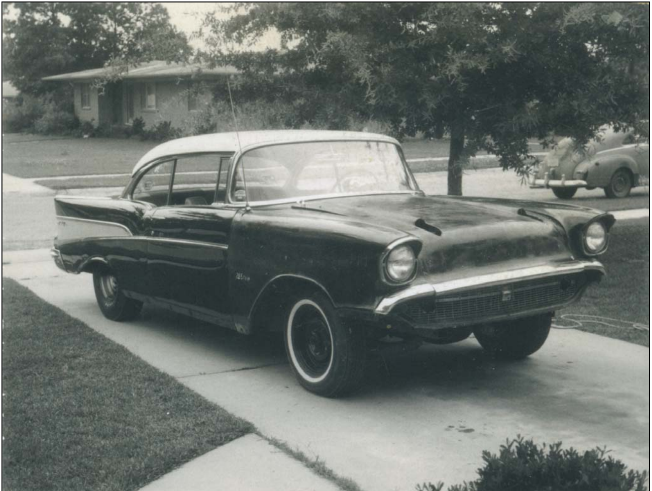
Figure 9: '57 Chevrolet with Fiberglas Hood and Fender The fiberglas hood and fender soon after installation. The chrome strip had not been installed yet. Note the "265" on the front fender behind the front wheel.
