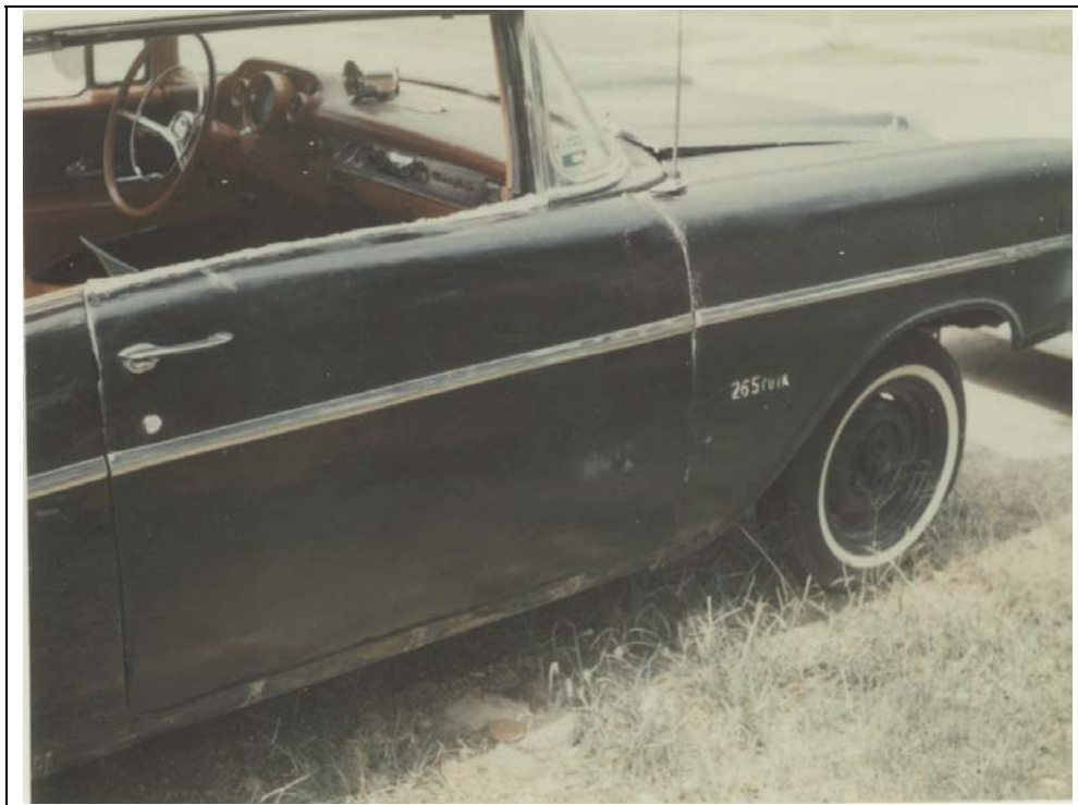
Figure 17: Fiberglas Door during Installation The door was trial fitted to the car. The vent window had not been installed yet.
