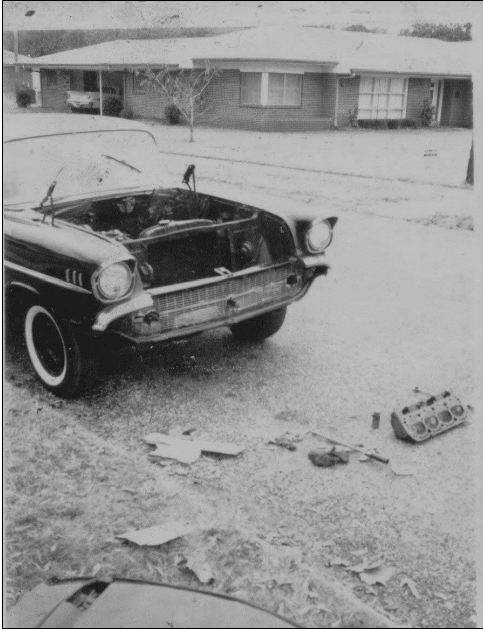
Figure 7: '57 Chevrolet Head Gasket Replacement The '57 is shown at my home in El Dorado on Ripley Avenue. The steel shim head gaskets were prone to leak probably because the heads and the block should have been surfaced. The hood was removed to make it easier to get to the engine.
